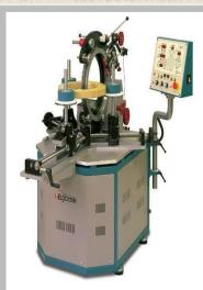
Maximum Wire Size:7AWG (3.66 mm)Minimum Wire Size:38AWG (0.1m mm) Maximum Coil O.D: 17.00" (431.3 mm) Minimum Coil O.D: 3.0"(76.2mm) Minimum Coil I.D: 0.5"(12.7mm) Maximum Coil Height: 7.0 - (177.6 mm)
