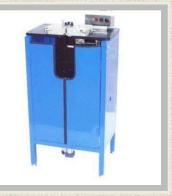
Maximum wire size: 2.0mm Minimum Wire Size: 0.3mm MaximumO.D: 60mm Minimum O.D: 15mm Minimum I.D: 5mm Minimum Core Height: 50mm Choices of 4 hooks Machineis operated by foot pedal which is easy to use
